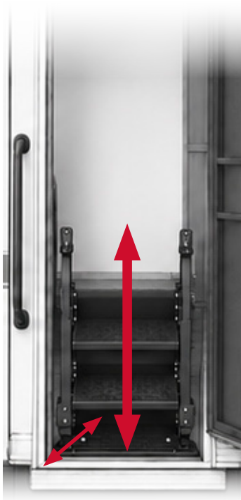
3-Step Extended Rise and Run Depth: 18.75" Height: 49.375"
