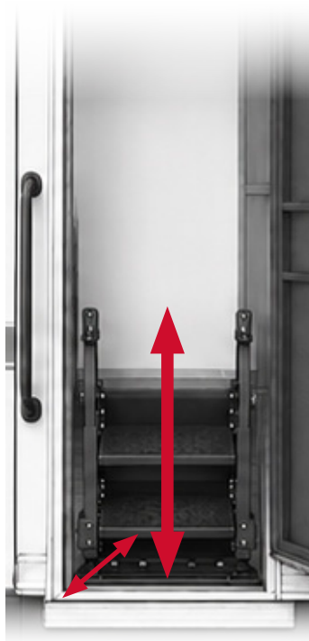
3-Step Standard Rise and Run Depth: 17.25" Height: 44.875"
